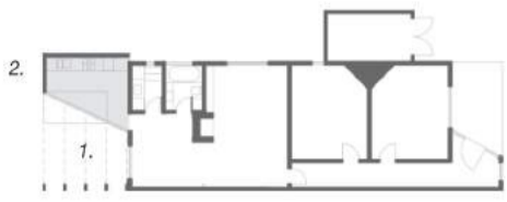
Plan of St Kilda East, new addition show in grey 1. forecourt deck 2. rear informal deck
