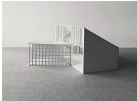
Study model at 1:50 of the new addition; structure, and bookshelves are shown.
